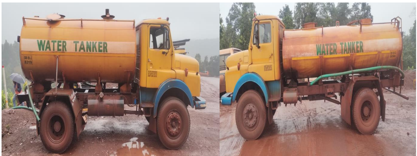
Photo-2 Mobile Water sprinkler tanker for dust suppression.
