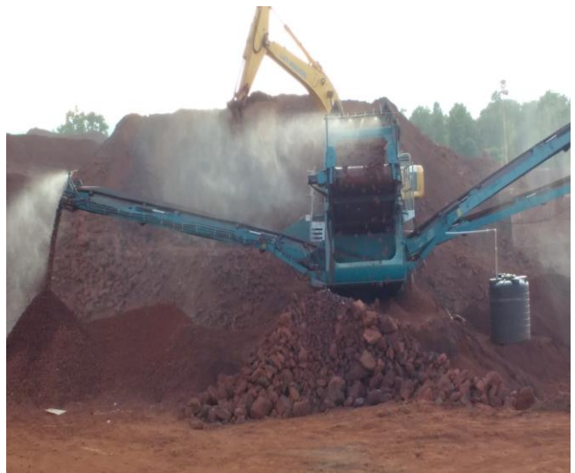
Photo-3 Mobile screen Plant Equipped with dry fog system for dust suppression
